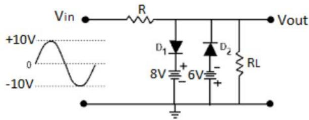
5. Sketch the output waveforms for the circuit shown below for  $V_i = 10 \sin(314t)$  assuming
